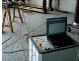
Fig. 8: CDS measurement in a high voltage laboratory
