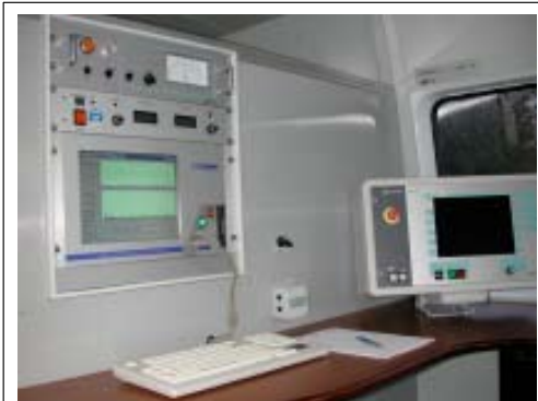
IPC with integrated PD Measuring System and HV -Source
