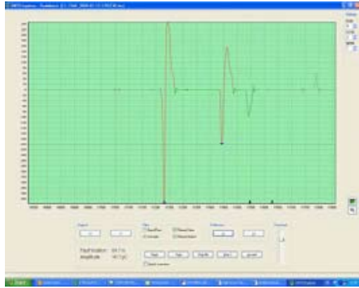
Figure 4: Wavelet filter applied to the reflection of fig. 1
