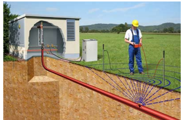
Pinpoint Location of a sheath fault
