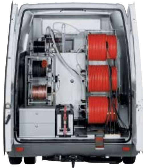
Test van with 3 single phase HV cables
