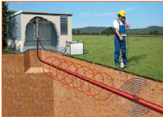
Fault location with SWG and Digiphone
